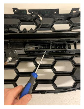
Check light bar is firmly in place and cannot move, install wiring and re fit grille to vehicle.
