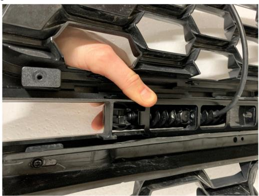
Once you have sandwiched the grille and tightened fitting as much as can be done from the outside of the grille, check fully tight from inside of grille.
